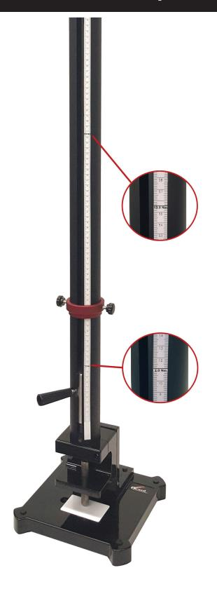
Q-Card's Resistance to Impact fixture is designed to determine a card's resistance to impact per ANSI, Mastercard® CQM and ISO standards.
